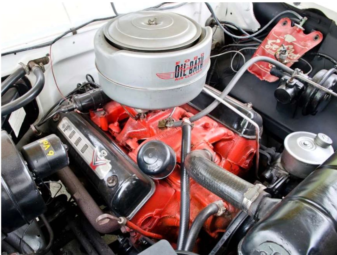
1955 Ford Y-block V-8 272-cid 162-hp U-code Engine w/ Dual Exhaust
